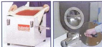
The FlexWall® feeder is well known to provide the fastest and easiest means of emptying, cleaning, and reassembling of any screw feeder. The internally agitated twin screw feeder has an optional easy access clean out panel.
